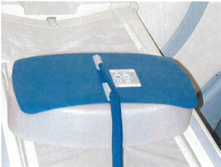
FIGURE 3. Experimental set-up used to evaluate artifacts for the Arctic Sun, Energy Transfer Pad. The Arctic Sun, Energy Transfer Pad was placed on the outside of a copper sulfate phantom to simulate its intended in vivo use. The phantom with the Arctic Sun, Energy Transfer Pad was the subjected to MRI at 3-Tesla using three different pulse sequences.
