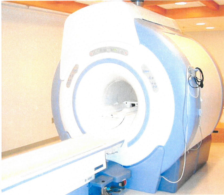
FIGURE 2. The 3-Tesla MR system (General Electric Healthcare, Milwaukee, WI) used for MRI testing of the Arctic Sun, Energy Transfer Pad.
