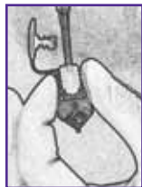
Add sample to SmartCycler tube and place in Smartcycler Instrument
