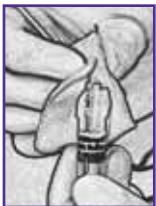
Break swab in sample buffer and transfer to lysis tube
