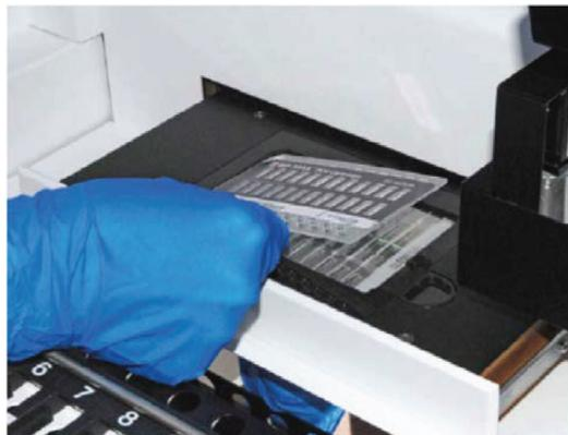
**Figura 2:** caricare le BD MAX PCR Cartridges.
