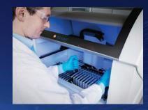
Load the Sample Buffer Tubes, racks, and PCR cartridges.
