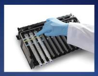
Assemble unitized reagent strips with extraction and PCR reagents.
