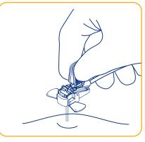
3 Insert needle perpendicular to the port septum.
