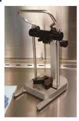
2 Remove the vial cap and disinfect per facility protocol. Place the vial on the assembly fixture base between the slide clamps.
