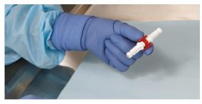
2 Engage the syringe units to the connectors by pushing each injector onto the connection interface until the two pieces snap together.
