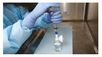
Disengage syringe unit 1 from the vial assembly by pulling the injector straight back from the connection interface.
