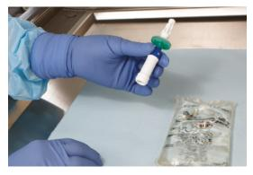
2 Engage the injector of the disc filter assembly to the connection interface on the infusion adapter by pushing the injector straight onto the connection interface until the two pieces snap together.
