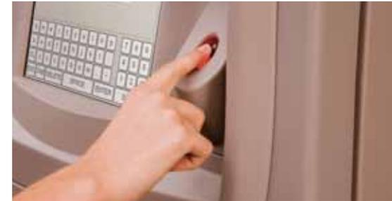
The optional BioID fingerprint identification system confirms user identity via fingerprint verification for login.
