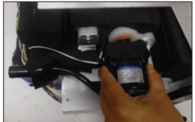
Fig. 8-47 Monter pumpen igen (trin 6) (to visninger)
