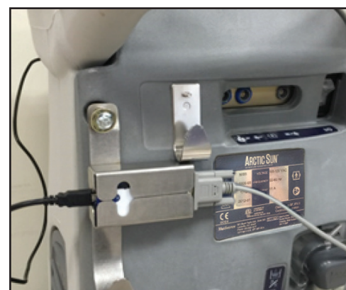
Fig. 8-74 Insert TIM and connect cables (Steps 3-5)
