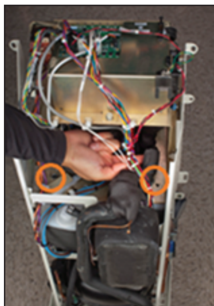
Fig. 8-17 Remove two bolts (Step 2)
