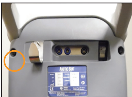
Fig. 8-72 Remove bolt (Step 1)
