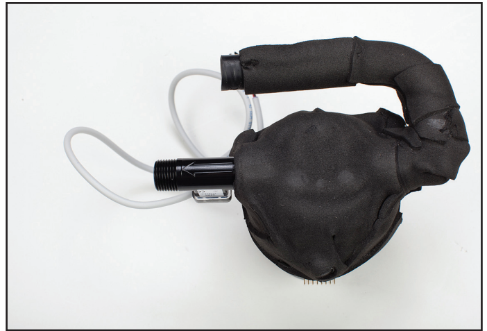
Fig. 8-53 Flowmeter with arrow indicating direction of flow; same direction as Circulation Pump output
