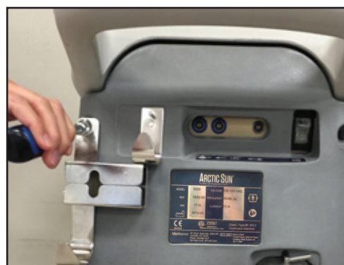
Fig. 8-73 Secure bracket (Step 2)
