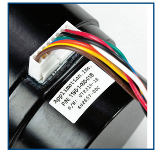
Fig. 8-32 Illustration of pump connector prior to being connected (above), connected but seated incorrectly with one pin exposed (below left), and seated correctly (below right)
