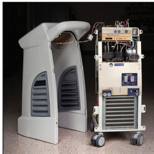
Fig. 8-13 Shell separated from internal components
