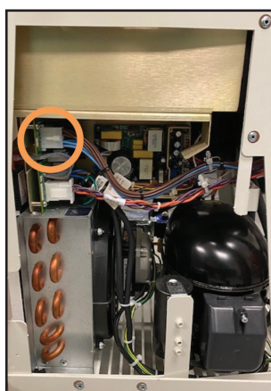
Fig. 7-4 Location of connector
