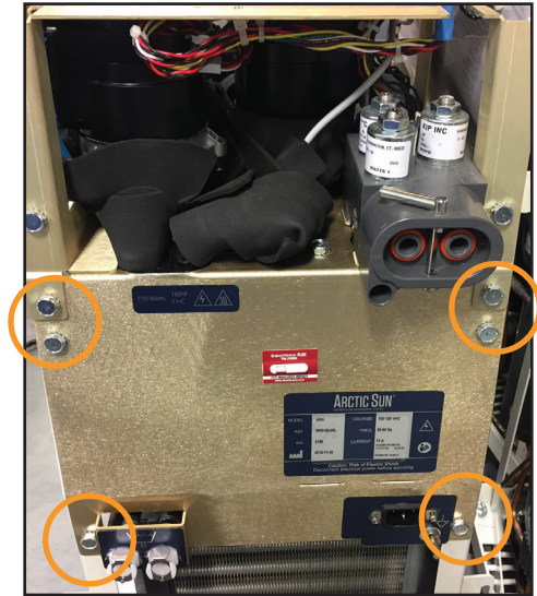
Fig. 8-36 Remove six bolts (Step 3)
