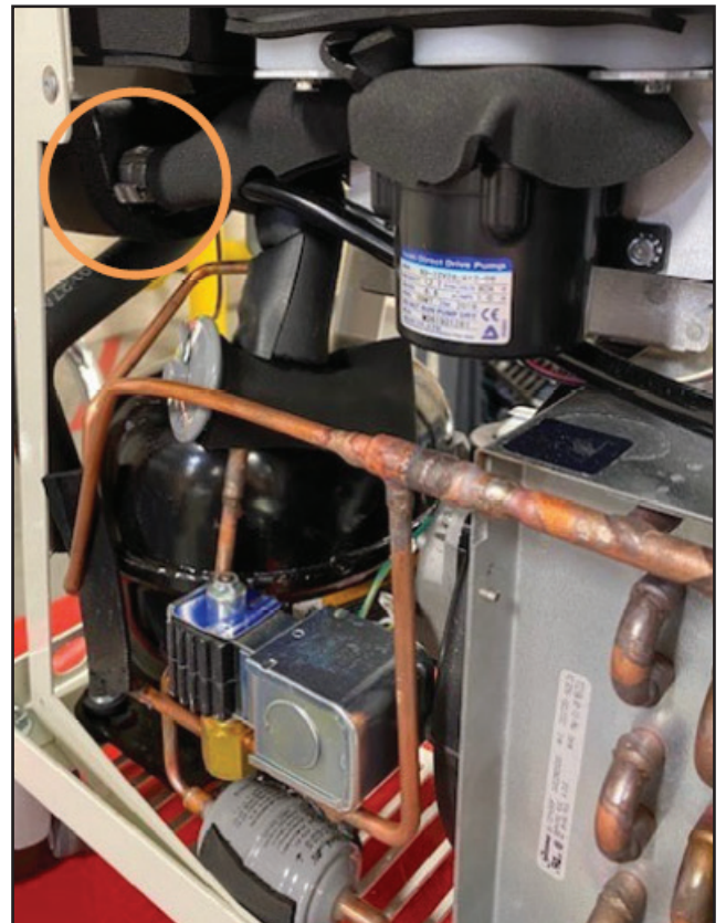
Fig. 8-22 Disconnect two clamps (Step 3- DC pump)
