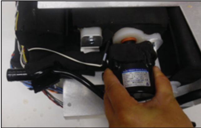
Fig. 8-47 Reinstall pump (Step 6) (two views)
