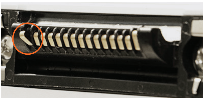
IUI connector with bent pin
