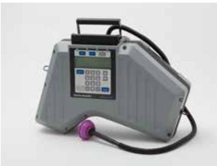
Figure 3 Thermo Scientific MIRAN SapphIRe analyzer.
