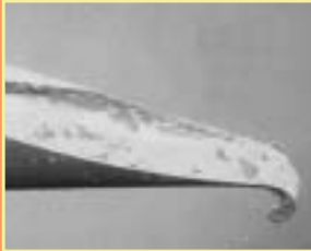
Tip damage caused by re-use
