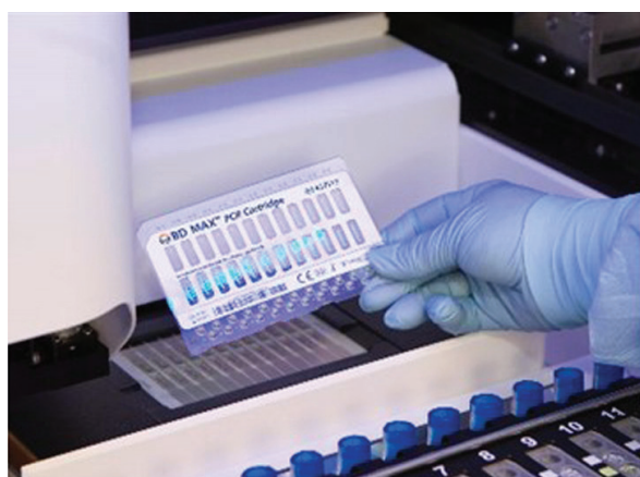
Figure 2: Load BD MAX PCR Cartridges.
